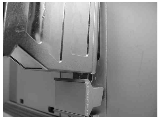
FIGURE 11. The slide lock has clicked into place, but is not secure on both posts. Do not permit this to happen.
