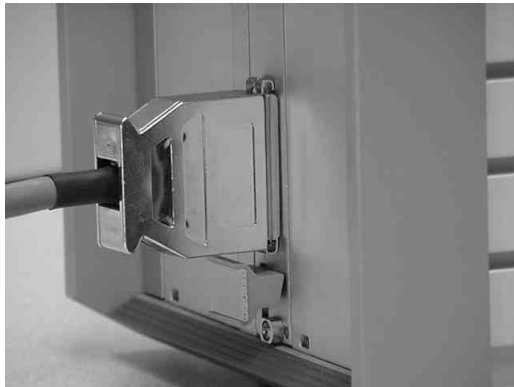
FIGURE 8. The Service Module cable is attached properly but not yet locked down. Note the loop at the top of the connector.
