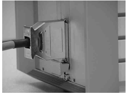
FIGURE 9. The Service Module cable is now properly locked in place. Note the new positions of the loops of the slide lock.
